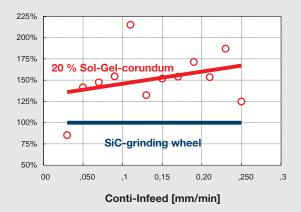
Diagram 2: Comparison of the G-ratio [cm<sup>3</sup>/cm<sup>3</sup>]
