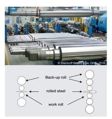
In addition to the mechanical equipment, the selection of the process parameters adapted to the grinding wheel specification is an essential step to meet the required dimensional needs, create the surface finish of the rolls and to achieve a cost-effective process management.
