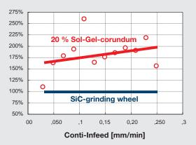
**Diagram 1:** Comparison of the specific machining performance [cm³/min/kW]
