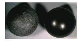
Ball material:  $Si_3N_4$ 300 pcs Charge: 180 µm Stock removal: Grinding time: 3,5 h Stock removal rate: 51 µm/h Pressing plate: steel
